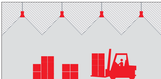
Warehouse with 300 lx
