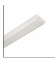
optical accessories, for Monsun®, enclosure, of PMMA, inner prismatic structure, for 2 x T16 | T26 28/36W, length: 1.271 mm, width: 130 mm
