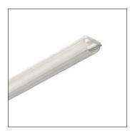
optical accessories, for Monsun®, enclosure, of PMMA, inner prismatic structure, for 1 x T16 | T26 28/36/54W, length: 1.271 mm, width: 84 mm
