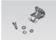
Universal luminaire suspension for wire ( \phi \leq 4.5\text{mm} ) or chain (inner \phi \geq 7\text{mm} ) Load capacity: 25kg
