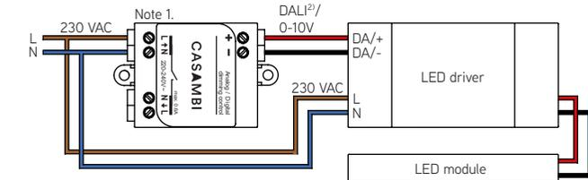
**Wiring diagram, DALI or 1-10V drivers powered through external relay**
