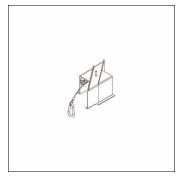
Silica®, ceiling mounting element, installation type: recessed, of aluminium/iron, length: 140 mm, width: 73 mm, height: 82mm, retaining cord, certification: CE, packaging unit: 1 piece
