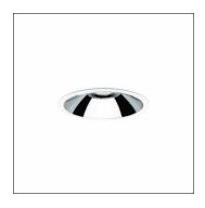
Lunis 21, XL, downlight, of PC, light emission: direct distribution, LED rated luminous flux: 2.180lm, light colour: 830, control gear: ECG, with terminal, 3-pole, mains connection: 220..240V, AC, housing, round, of diecast aluminium, traffic white (RAL 9016), diameter: 213mm, protection rating (complete): IP20, protection rating (on room side): IP54, insulation class (complete): insulation class II (safety insulation), certification: CE, impact resistance: IK02, packaging unit: 1 piece
