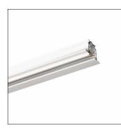
AX T, 3-phase track, installation type: recessed, mains connection: 220..240V/380..400V, AC, of extruded aluminium section, coated, white, length: 2.000 mm, width: 32 mm, height: 33mm, protection rating (complete): IP20, insulation class (complete): insulation class I (protective earthing), certification: CE, ENEC, packaging unit: 1 piece
