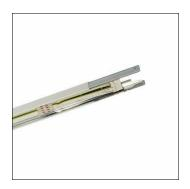
Modario®, trunking rail, of sheet steel, coated, pure white, 1-length, length: 1.196 mm, width: 58 mm, height: 43mm, through-wiring: 10x 2.5mm², with terminal, 10-pole, max. 2.5mm², protection rating (complete): for IP20/IP40 protection rating, insulation class (complete): insulation class I (protective earthing), certification: CE, ENEC, VDE, standard: EN 60598, packaging unit: 1 piece
