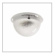
electrics components group, for Small Bell, control gear: ECG Plus, LED luminous flux: 1.660 lm, colour temperature: 3000K, mains connection: 230..240V, AC, 50/60Hz, start of lifetime: 13 W, end of service life: 14 W, reduction: 7 W, primary light characteristic: asymmetric, primary optical cover: enclosure, of PMMA, transparent structured, gear tray with cover, insulation class (complete): insulation class II (safety insulation), certification: CE, ENEC, VDE
