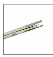
Modario<sup>®</sup> IP64, trunking rail, of sheet steel, galvanised, coated, pure white, 3length, length: 4.485 mm, width: 58 mm, height: 43mm, through-wiring: 10x 2.5mm<sup>2</sup>, with terminal, 10-pole, max. 2.5mm<sup>2</sup>, protection rating (complete): for IP64 protection rating, insulation class (complete): insulation class I (protective earthing), certification: CE, ENEC, VDE, standard: EN 60598, packaging unit: 1 piece
