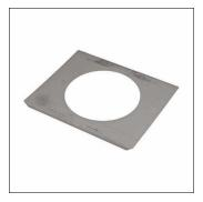
Lunis 11 R, mounting element, installation type: recessed, mounting plate, Module 625, of sheet steel, galvanised, for 5LR610..., for supporting luminaire weight on supporting structure, length: 620mm, width: 500mm, height: 25mm, packaging unit: 1 piece
