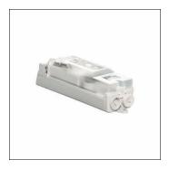
cable junction box, for 3 cables to 5x 16mm², L1/L2/L3/L4/PE(N), 3x E14, cable junction box, of plastic, shock-resistant, inner mast diameter: from 89mm, protection rating (complete): IP54, insulation class (complete): insulation class II (safety insulation), certification: CE, VDE, packaging unit: 1 piece
