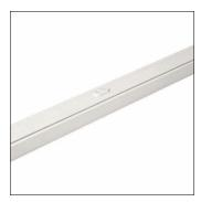
housing accessories, for Modario® IP64, trunking rail, additional feed-in/-out, of steel, galvanised, coated, pure white, 5x system unit, length: 1.495 mm, width: 58 mm, height: 43mm, through-wiring: 10x 2.5mm², protection rating (complete): for IP64 protection rating, insulation class (complete): insulation class I (protective earthing), certification: CE, UKCA, packaging unit: 1 piece
