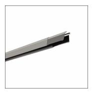
Licross®, trunking rail, of sheet steel, galvanised, coil coated, metallic grey (RAL 9006), length: 4.500 mm, width: 64 mm, height: 67mm, through-wiring: 9x 2.5mm², protection rating (complete): maximum IP64, depends on used inserts and accessories, insulation class (complete): insulation class I (protective earthing), certification: CE, UKCA, LABS conformity tested according to VDMA 24364:2018-05, packaging unit: 1 piece
