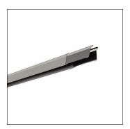
Licross®, trunking rail, of sheet steel, galvanised, coil coated, metallic grey (RAL 9006), length: 3.000 mm, width: 64 mm, height: 67mm, through-wiring: 9x 2.5mm², protection rating (complete): maximum IP64, depends on used inserts and accessories, insulation class (complete): insulation class I (protective earthing), certification: CE, UKCA, LABS conformity tested according to VDMA 24364:2018-05, packaging unit: 1 piece
