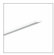
DUS® IP20DUS® mounting rail, blank cover, installation type: surface-mounted, blank cover, of plastic, uncoated, white, can be cut to suit, length: 1.535mm, width: 60mm, height: 20mm, protection rating (complete): IP20, packaging unit: 1 piece
