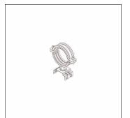
Monsun® 11/21, pipe clip fixing, installation type: surface-mounted, mounting set, consisting of each 2x pipe clamps of galvanised steel with rubber inlay, cylinder head screw, mounting clip for luminaire of V2A and 2x fixing reinforcement of UV-stabilised PC, clamping range: for pipe diameter 2", packaging unit: set of 2
