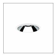
Lunis 21, XL, downlight, of PC, light emission: direct distribution, LED rated luminous flux: 3.360lm, light colour: 830, control gear: ECG DALI, with terminal, 5-pole, mains connection: 220..240V, AC, housing, round, of diecast aluminium, traffic white (RAL 9016), diameter: 213mm, protection rating (complete): IP20, protection rating (on room side): IP54, insulation class (complete): insulation class II (safety insulation), certification: CE, impact resistance: IK02, packaging unit: 1 piece
