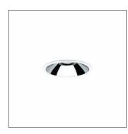
Lunis 21, L, downlight, of PC, light emission: direct distribution, LED rated luminous flux: 1.670lm, light colour: 830, control gear: ECG, with terminal, 3-pole, mains connection: 220..240V, AC, housing, round, of diecast aluminium, traffic white (RAL 9016), diameter: 162mm, protection rating (complete): IP20, protection rating (on room side): IP54, insulation class (complete): insulation class II (safety insulation), certification: CE, impact resistance: IK02, packaging unit: 1 piece
