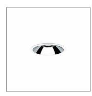
Lunis 21, L, downlight, of PC, light emission: direct distribution, LED rated luminous flux: 1.670lm, light colour: 830, control gear: ECG DALI, with terminal, 5-pole, mains connection: 220..240V, AC, housing, round, of diecast aluminium, traffic white (RAL 9016), diameter: 162mm, protection rating (complete): IP20, protection rating (on room side): IP54, insulation class (complete): insulation class II (safety insulation), certification: CE, impact resistance: IK02, packaging unit: 1 piece
