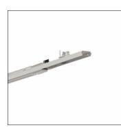
Modario<sup>®</sup>, track adapter insert, with plug, 5-pole, with phase selection, for trunking rail, 10-core, mains connection: 230/400V, track adapter insert, of sheet steel, coil coated, metallic grey (RAL 9006), 2x system unit, max. weight load 5kg, length: 598mm, width: 48mm, protection rating (complete): for IP20 protection rating, insulation class (complete): insulation class I (protective earthing), certification: CE, packaging unit: 1 piece
