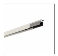
Licross®, trunking rail, of sheet steel, galvanised, coil coated, white, length: 1.500 mm, width: 64 mm, height: 67mm, through-wiring: 11x 2.5mm<sup>2</sup>, protection rating (complete): maximum IP64, depends on used inserts and accessories, insulation class (complete): insulation class I (protective earthing), certification: CE, UKCA, LABS conformity tested according to VDMA 24364:2018-05, packaging unit: 1 piece
