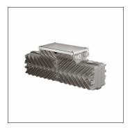
Sirius®, ECG unit, 3/4-pole (3/4G), max. 2.5mm² + 2xRJ45 (DMX In/Out), control gear: ECG, with terminal, mains connection: 220..240V/380..415V, AC, 50/60Hz, with system connector or terminal, ECG unit, of diecast aluminium, powder-coated, Siteco® metallic grey (DB 702S), length: 635mm, width: 181mm, height: 247mm, protection rating (complete): IP66, insulation class (complete): insulation class I (protective earthing), certification: CE, ENEC, packaging unit: 1 piece
