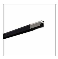
Licross®, trunking rail, of sheet steel, galvanised, coil coated, matt jet black (RAL 9005), length: 4.500 mm, width: 64 mm, height: 67mm, through-wiring: 11x 2.5mm², protection rating (complete): maximum IP64, depends on used inserts and accessories, insulation class (complete): insulation class I (protective earthing), certification: CE, UKCA, LABS conformity tested according to VDMA 24364:2018-05, packaging unit: 1 piece
