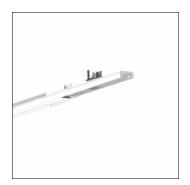
Modario®, track adapter insert, control gear: ON/OFF, with plug, 5-pole, with phase selection, for trunking rail, 5 or 10-core, mains connection: 230/400V, track adapter insert, of sheet steel, coil coated, pure white, 4x system unit, max. weight load 5kg, length: 1.196mm, width: 48mm, protection rating (complete): for IP20 protection rating, insulation class (complete): insulation class I (protective earthing), certification: CE, packaging unit: 1 piece
