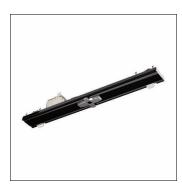
Licross<sup>®</sup>, rail insert, adapter, with plug, 5-pole, with phase selection, mains connection: 230V, AC, 50/60Hz, terminal,5-pole, max. 2.5mm<sup>2</sup>, multi adapter, of sheet steel, coil coated, matt jet black (RAL 9005), for IP20/IP40 protection rating, length: 500mm, width: 64mm, height: 68mm, multifunctional insert, protection rating (complete): IP20, insulation class (complete): insulation class I (protective earthing), certification: CE, UKCA, packaging unit: 1 piece
