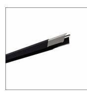
Licross<sup>®</sup>, trunking rail, of sheet steel, galvanised, coil coated, matt jet black (RAL 9005), length: 4.500 mm, width: 64 mm, height: 67mm, protection rating (complete): maximum IP64, depends on used inserts and accessories, insulation class (complete): insulation class I (protective earthing), certification: CE, UKCA, LABS conformity tested according to VDMA 24364:2018-05, packaging unit: 1 piece
