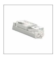
cable junction box, for 3 cables to 5x 16mm<sup>2</sup>, L1/L2/L3/N/PE, 2x E14, cable junction box, of plastic, shock-resistant, inner mast diameter: from 89mm, protection rating (complete): IP54, insulation class (complete): insulation class II (safety insulation), certification: CE, VDE, packaging unit: 1 piece
