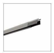
Licross®, trunking rail, of sheet steel, galvanised, coil coated, metallic grey (RAL 9006), length: 4.500 mm, width: 64 mm, height: 67mm, through-wiring: 11x 2.5mm², protection rating (complete): maximum IP64, depends on used inserts and accessories, insulation class (complete): insulation class I (protective earthing), certification: CE, UKCA, LABS conformity tested according to VDMA 24364:2018-05, packaging unit: 1 piece
