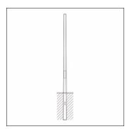
mast, mast, conical round, of steel, galvanised, height: 4.5m, spigot size: 60mm (post-top), planted section: h= 800mm / Ø= 134mm, standard: DIN EN 40, packaging unit: 1 piece
