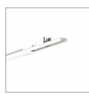
Modario<sup>®</sup>, track adapter insert, control gear: DALI, with plug, 5-pole, with phase selection, for trunking rail, 10-core, mains connection: 230/400V, track adapter insert, of sheet steel, coil coated, pure white, 4x system unit, max. weight load 5kg, length: 1.196mm, width: 48mm, protection rating (complete): for IP20 protection rating, insulation class (complete): insulation class I (protective earthing), certification: CE, packaging unit: 1 piece
