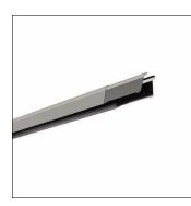
Licross<sup>®</sup>, trunking rail, of sheet steel, galvanised, coil coated, metallic grey (RAL 9006), length: 3.000 mm, width: 64 mm, height: 67mm, protection rating (complete): maximum IP64, depends on used inserts and accessories, insulation class (complete): insulation class I (protective earthing), certification: CE, UKCA, LABS conformity tested according to VDMA 24364:2018-05, packaging unit: 1 piece
