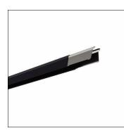
Licross<sup>®</sup>, trunking rail, of sheet steel, galvanised, coil coated, matt jet black (RAL 9005), length: 3.000 mm, width: 64 mm, height: 67mm, through-wiring: 11x 2.5mm<sup>2</sup>, protection rating (complete): maximum IP64, depends on used inserts and accessories, insulation class (complete): insulation class I (protective earthing), certification: CE, UKCA, LABS conformity tested according to VDMA 24364:2018-05, packaging unit: 1 piece
