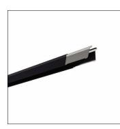
Licross<sup>®</sup>, trunking rail, of sheet steel, galvanised, coil coated, matt jet black (RAL 9005), length: 4.500 mm, width: 64 mm, height: 67mm, through-wiring: 14x 2.5mm<sup>2</sup>, protection rating (complete): maximum IP64, depends on used inserts and accessories, insulation class (complete): insulation class I (protective earthing), certification: CE, UKCA, LABS conformity tested according to VDMA 24364:2018-05, packaging unit: 1 piece
