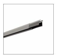
Licross®, trunking rail, of sheet steel, galvanised, coil coated, metallic grey (RAL 9006), length: 3.000 mm, width: 64 mm, height: 67mm, through-wiring: 14x 2.5mm², protection rating (complete): maximum IP64, depends on used inserts and accessories, insulation class (complete): insulation class I (protective earthing), certification: CE, UKCA, LABS conformity tested according to VDMA 24364:2018-05, packaging unit: 1 piece
