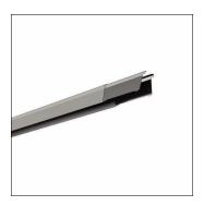
Licross®, trunking rail, of sheet steel, galvanised, coil coated, metallic grey (RAL 9006), length: 1.500 mm, width: 64 mm, height: 67mm, through-wiring: 14x 2.5mm², protection rating (complete): maximum IP64, depends on used inserts and accessories, insulation class (complete): insulation class I (protective earthing), certification: CE, UKCA, LABS conformity tested according to VDMA 24364:2018-05, packaging unit: 1 piece
