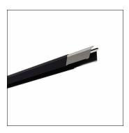
Licross®, trunking rail, of sheet steel, galvanised, coil coated, matt jet black (RAL 9005), length: 3.000 mm, width: 64 mm, height: 67mm, through-wiring: 14x 2.5mm², protection rating (complete): maximum IP64, depends on used inserts and accessories, insulation class (complete): insulation class I (protective earthing), certification: CE, UKCA, LABS conformity tested according to VDMA 24364:2018-05, packaging unit: 1 piece
