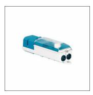
cable junction box, for 3 cables to 5x 16mm², L1/L2/L3/N/PE, 1x E14, cable junction box, of plastic, shock-resistant, inner mast diameter: from 84mm, protection rating (complete): IP44, insulation class (complete): insulation class II (safety insulation), certification: CE, packaging unit: 1 piece
