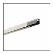
Licross®, trunking rail, of sheet steel, galvanised, coil coated, white, length: 4.500 mm, width: 64 mm, height: 67mm, through-wiring: 11x 2.5mm², protection rating (complete): maximum IP64, depends on used inserts and accessories, insulation class (complete): insulation class I (protective earthing), certification: CE, UKCA, LABS conformity tested according to VDMA 24364:2018-05, packaging unit: 1 piece
