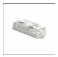
cable junction box, for 3 cables to 5x 16mm², L1/L2/L3/L4/PE(N), 2x E14, cable junction box, of plastic, shock-resistant, inner mast diameter: from 89mm, protection rating (complete): IP54, insulation class (complete): insulation class II (safety insulation), certification: CE, VDE, packaging unit: 1 piece
