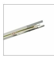
Modario<sup>®</sup> IP64, trunking rail, of sheet steel, galvanised, coated, pure white, 2length, length: 2.990 mm, width: 58 mm, height: 43mm, through-wiring: 10x 2.5mm<sup>2</sup>, with terminal, 10-pole, max. 2.5mm<sup>2</sup>, protection rating (complete): for IP64 protection rating, insulation class (complete): insulation class I (protective earthing), certification: CE, ENEC, VDE, standard: EN 60598, packaging unit: 1 piece
