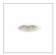
Lunis 31, midi, downlight, light control with reflector, light emission: direct distribution, LED rated luminous flux: 2.000lm, light colour: 830, mains connection: 220..240V, AC, 50/60Hz, housing, white, protection rating (complete): IP20, protection rating (on room side): IP54, insulation class (complete): insulation class II (safety insulation), certification: CE, packaging unit: 1 piece
