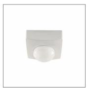
SITECO ConnectSensor-Head PC5-S, slave, local control - self-sufficient standalone sensors, central control - connection to lighting or building management, dimmable, installation type: slip-in mounting, installation location: on interface, of plastic, protection rating (complete): IP54, certification: CE, VDE, 1 x PIR movement sensor, 1 x light sensor, packaging unit: 1 piece
