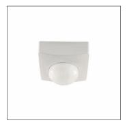
Siteco Connect Sensor-HeadSensor-Head PR1-M, master, local control, switchable, dimmable, installation type: slip-in mounting, installation location: on interface, of plastic, protection rating (complete): IP54, certification: CE, VDE, 1 x PIR movement sensor, 1 x light sensor, 1 x IR receiver, packaging unit: 1 piece
