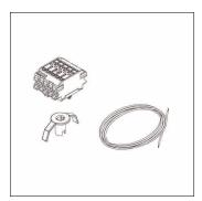
Monsun® 11/21, through-wiring, installation type: recessed, through-wiring set,3-core, 2.5mm², cable length: 1,4m, terminal,3-pole, max. 2.5mm², with protective earth, insulation class (complete): insulation class I (protective earthing), packaging unit: 1 piece
