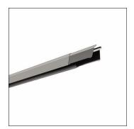
Licross®, trunking rail, of sheet steel, galvanised, coil coated, metallic grey (RAL 9006), length: 4.500 mm, width: 64 mm, height: 67mm, through-wiring: 7x 2.5mm², protection rating (complete): maximum IP64, depends on used inserts and accessories, insulation class (complete): insulation class I (protective earthing), certification: CE, UKCA, LABS conformity tested according to VDMA 24364:2018-05, packaging unit: 1 piece
