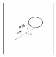
Vega® 11, wire suspension, ceiling sleeve, of steel, nickel-plated, wire, of steel, galvanised, fixing on luminaire side, of steel, galvanised, packaging unit: 1 piece
