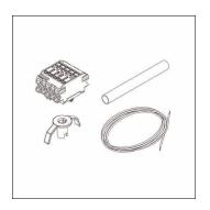
Monsun<sup>®</sup> 11/21, through-wiring, installation type: recessed, through-wiring set,5-core, 2.5mm<sup>2</sup>, cable length: 1,7m, terminal,5-pole, max. 2.5mm<sup>2</sup>, with protective earth, insulation class (complete): insulation class I (protective earthing), packaging unit: 1 piece
