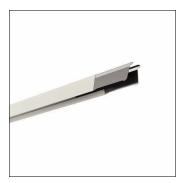
Licross®, trunking rail, of sheet steel, galvanised, coil coated, white, length: 1.500 mm, width: 64 mm, height: 67mm, through-wiring: 5x 2.5mm<sup>2</sup>, protection rating (complete): maximum IP64, depends on used inserts and accessories, insulation class (complete): insulation class I (protective earthing), certification: CE, UKCA, LABS conformity tested according to VDMA 24364:2018-05, packaging unit: 1 piece
